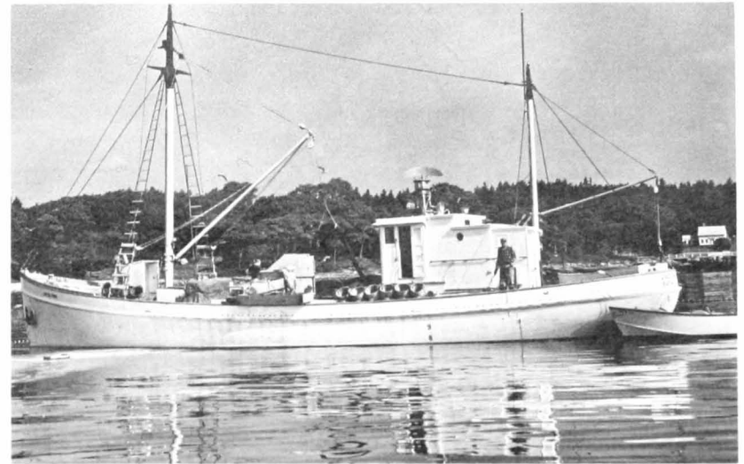
A sardine carrier. The herring — 2 years old and 7 inches long — are pumped into the carrier and lightly salted for the 6-hour trip to the factory. The ash-splint baskets beside the wheelhouse are used for collecting scales.
